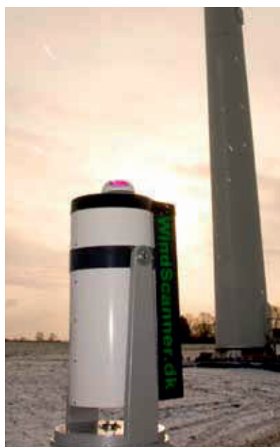
Short-range Windscanner situated in front of a test wind turbine at Risø DTU.
