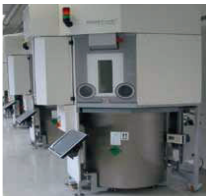
BBMRI includes a sample storage infrastructure. See here a hermetic semi-automated cryo-storage system.
