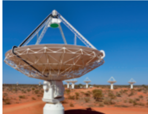
ASKAP: The CSIRO's Australian SKA Pathfinder (ASKAP) telescope, located at the Murchison Radio-astronomy Observatory (MRO) in Western Australia. ASKAP is composed of 36 antennas and is one of the precursor telescopes to the SKA.
