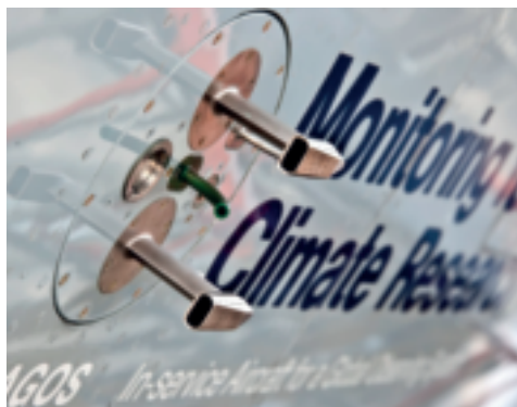
IAGOS Air Sampling Probes on the Lufthansa A340 Viersen. Source: Lufthansa
