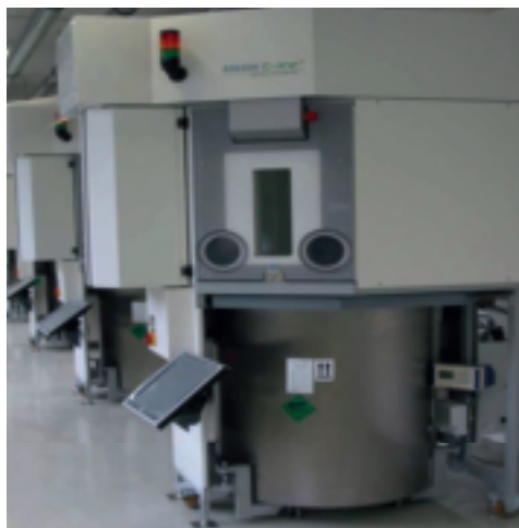
BBMRI includes a sample storage infrastructure. See here a hermetic semi-automated cryo-storage system.
